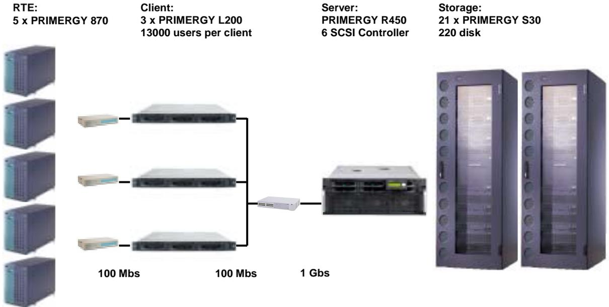
**Figure 2: Priced System Configuration PRIMERGY R450**
