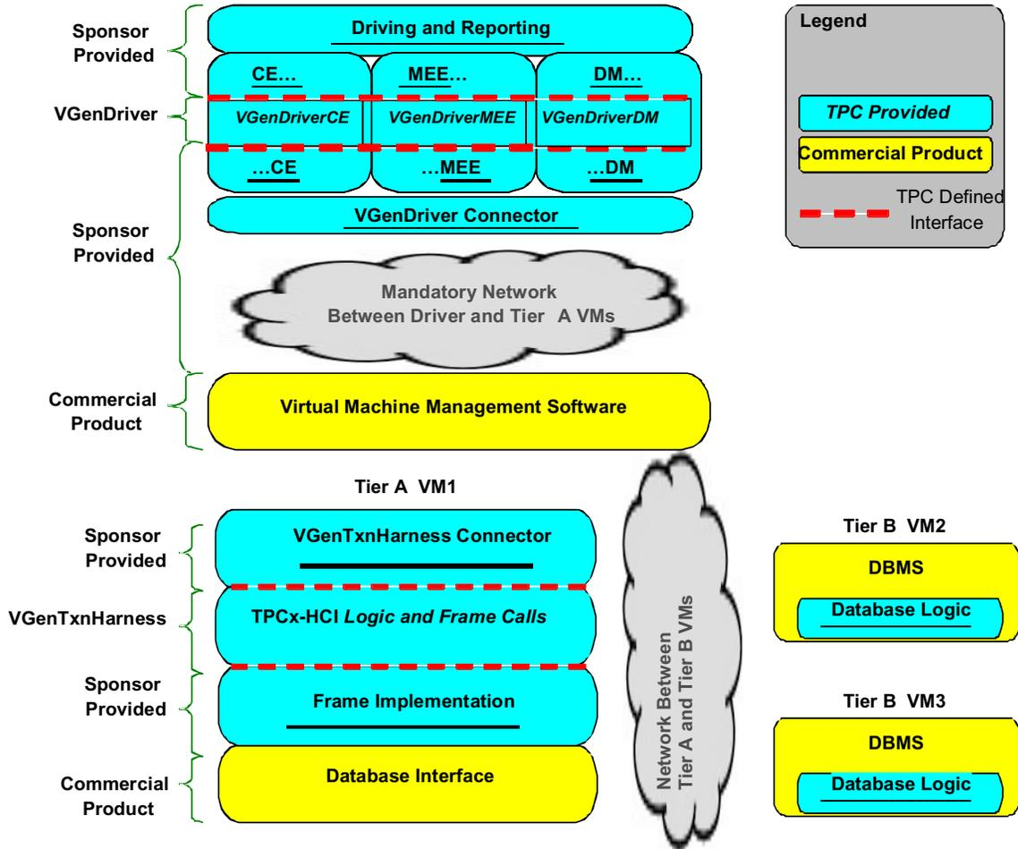
Figure 10.c - Functional Components of the Test Configuration
