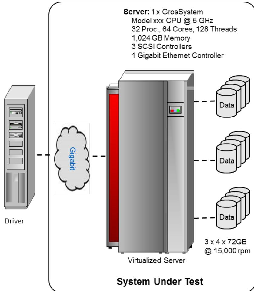
Figure 8a - Example of Measured Benchmark Configuration
