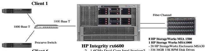
2 - 1.6GHz Dual Core Intel Itanium2 with 24MB iL3 Cache 192GB Memory
