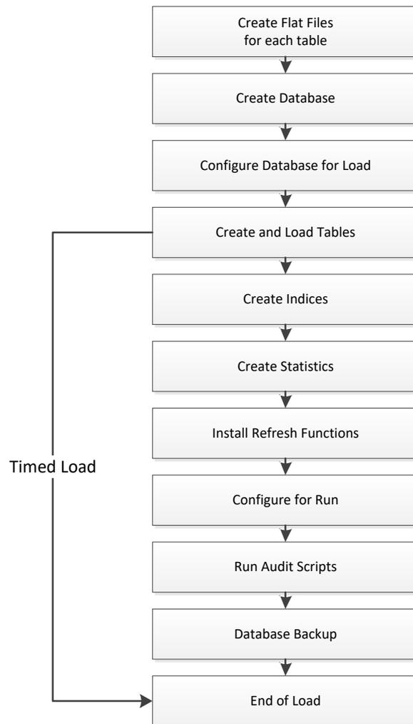
Figure 4.8: Block Diagram of Database Load Process
